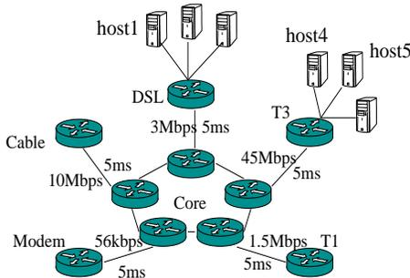
Fig. 1. Experimental topology on Emulab. The links in the core network are unmodified 100 Mbps Ethernet links.
